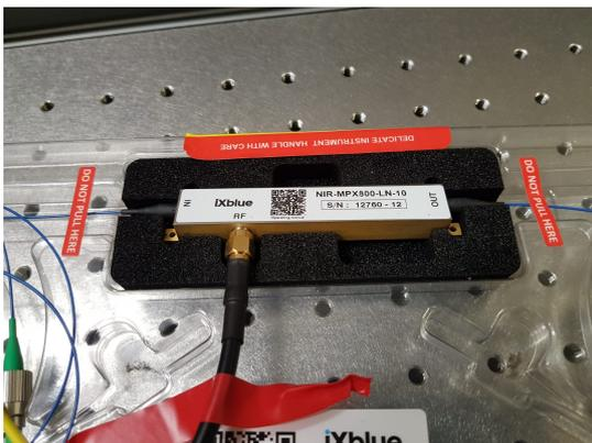
Figure 4.3: An image of the electro-optical modulator.
