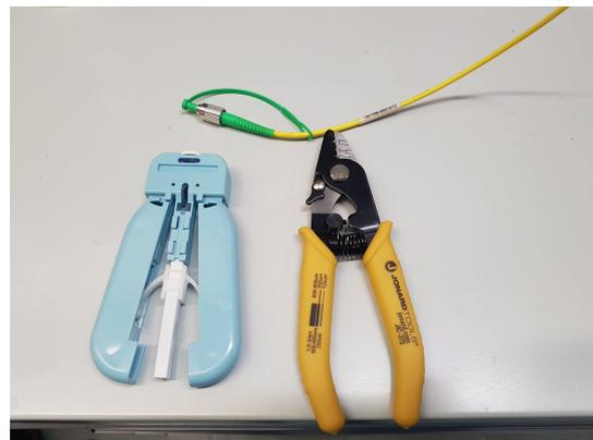
Figure 3.26: The tools necessary to strip an optical patch cable of its isolation, special pliers for the outside isolation (right) and a dedicated stripper for the inside one (left).
