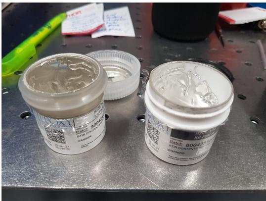
Figure 3.28: The two-component silver glue used.
