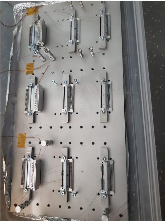
Figure 3.34: The fiber stockpile holder in which the fibers are placed when they arrive from the coating company.
