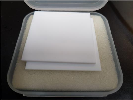
Figure 3.38: The Macor<sup>®</sup> Ceramic plates used in building the fiber holders for piezo isolation.
