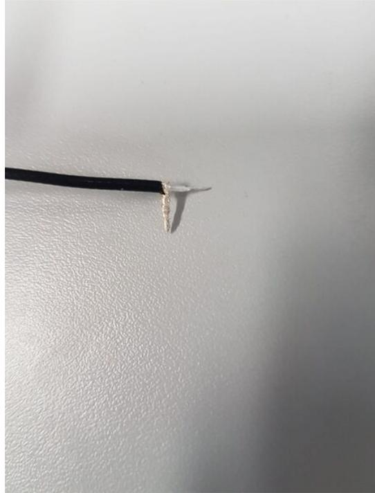
Figure 3.15: Cut rotation stage cable stripped of isolation and with twisted outer conductor.
