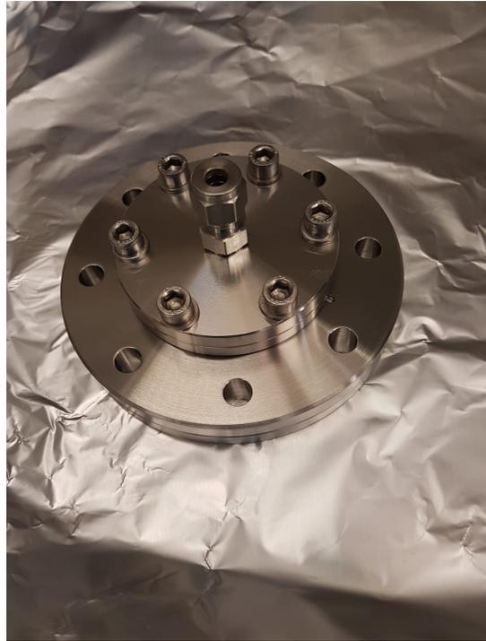
Figure 3.20: A Swagelok gas inlet repurposed as a fiber feedthrough.
