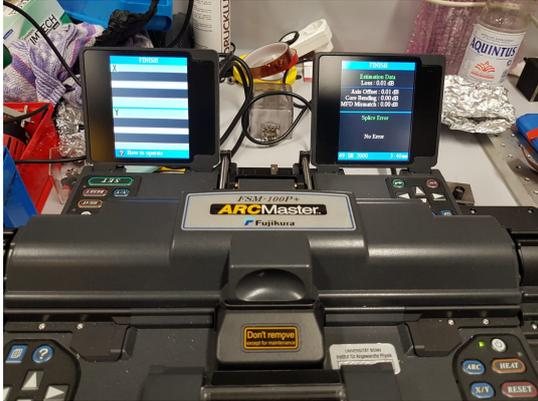
Figure 3.23: The “Fujikura ArcMaster FSM-100P+” splicer.
