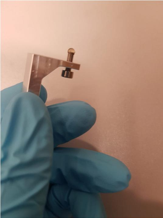
Figure 3.62: The L-piece with screw and UV-glove at its tip.
