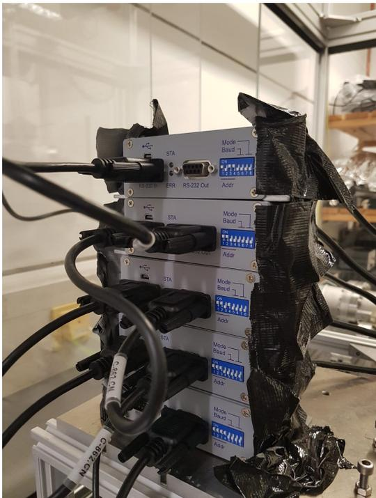
Figure 3.10: The whole translation stage controller stack in the daisy chain configuration. The individual controllers were connected to each other and one had to input their binary address in the daisy chain by switching their “Addr.”-buttons.
