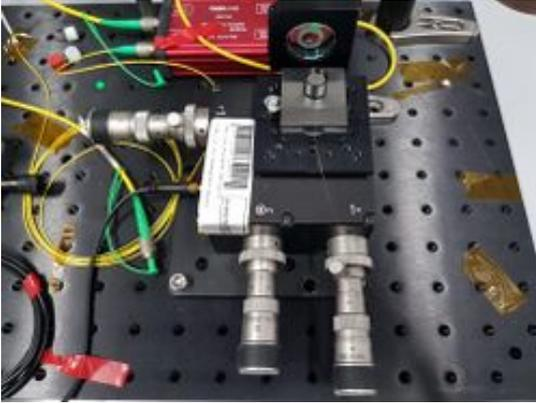
Figure 3.32: The basic mirror testing setup, consisting just of a fiber mirror, attached to a manual translation stage, and a mirror substrate.
