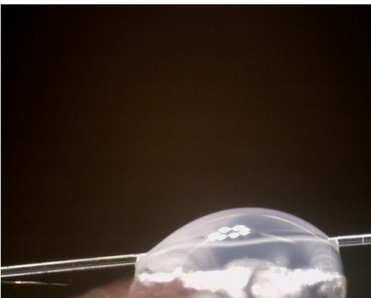
Figure 3.42: The UV-glue as it was applied to the piezo to fixate fiber1.
