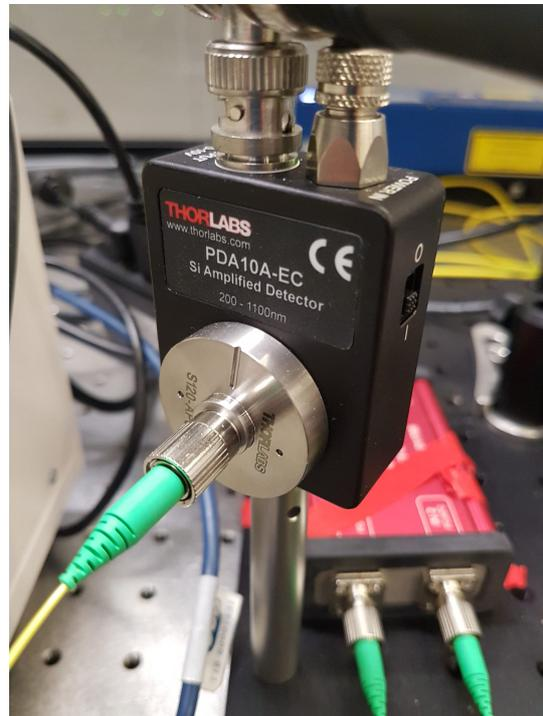
Figure 4.2: An image of the photo diode used in the experiment.
