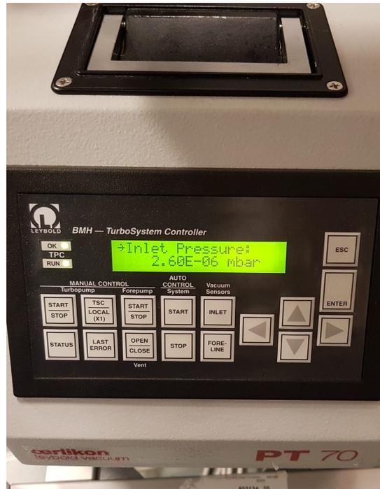
Figure 3.57: A pressure reading after two weeks of pumping with the turbopump of  $2.6 \cdot 10^{-6}$  mbar.
