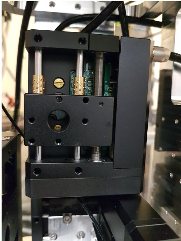
Figure 3.18: As stage 5 had to be mounted to stage 4, an aluminum connection block was necessary, the through holes of stage 5 were used with brass screws to interface it.
