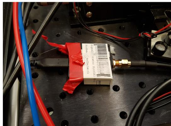
Figure 4.4: The function generator that drives the EOM.
