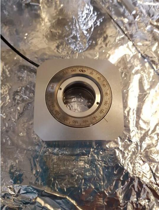
Figure 3.14: The rotation stage that will hold the mirror substrate for the experiment.
