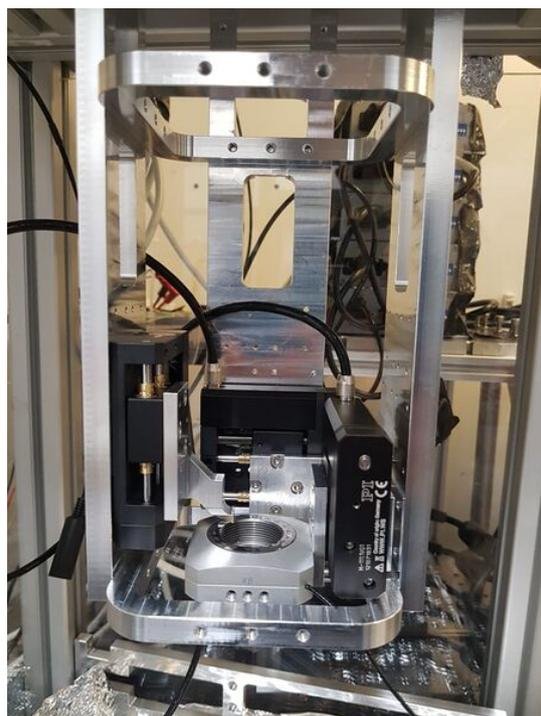
Figure 3.13: Complete assembly of the basic setups inner structure, now with the rotation stage attached.
