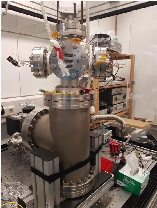
Figure 3.56: The inner setup was lowered into the vacuum chamber.
