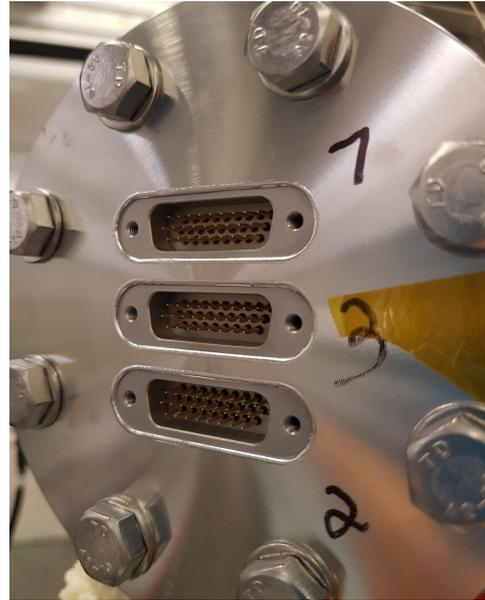
Figure 3.9: The custom translation stage feedthroughs.
