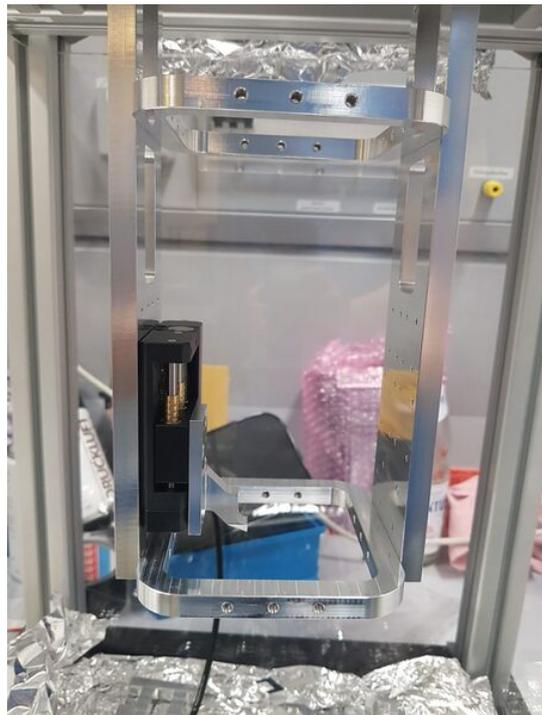
Figure 3.11: The inner aluminum structure with the first translation stage that will control the left fiber.
