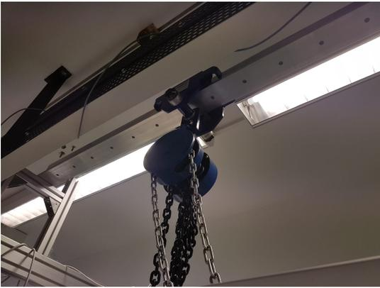
Figure 3.52: The rail and hoist used for inner structure transportation.
