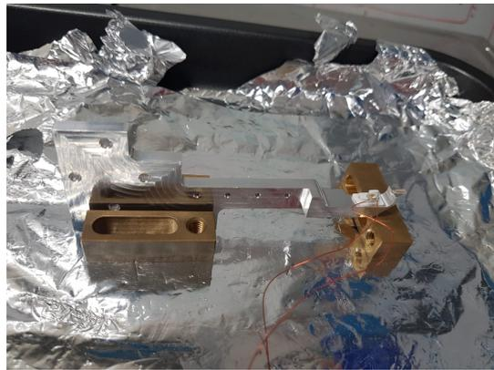
Figure 3.41: The second fiber holder that will place the second fiber above the mirror substrate as soon as the experimental setup is completed. Piezo and ferrule are visible on the right.
