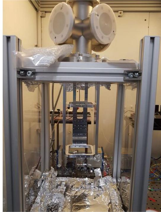
Figure 3.5: The basic outer support and protection structure with the inner frame for stage attachment partially assembled.
